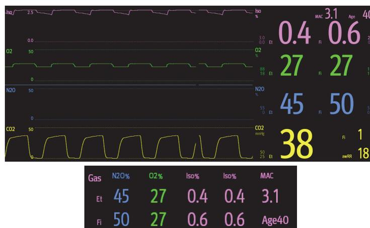
The AG module can send waves and numerics for all measured anesthetic gases for display on the monitor, including:
